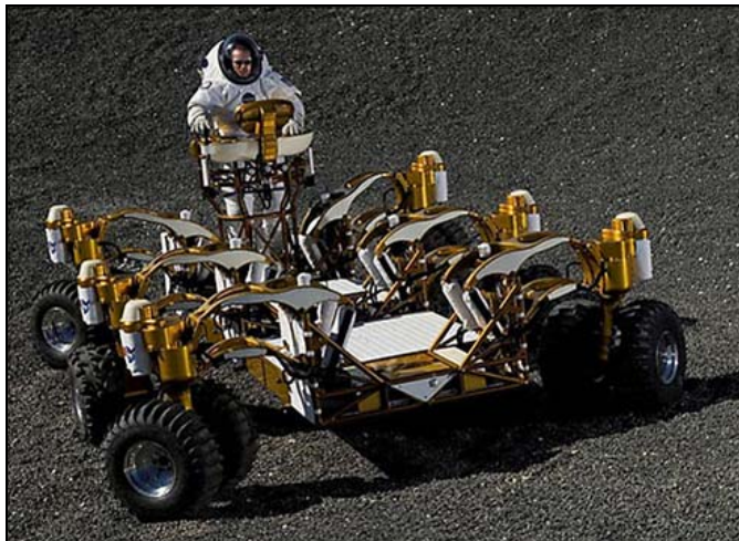
The Chariot Lunar Truck is one idea for a vehicle equal to the lunar terrain. Each of the six wheels pivot in any direction, and two turrets allow the astronauts to rotate 360°.
