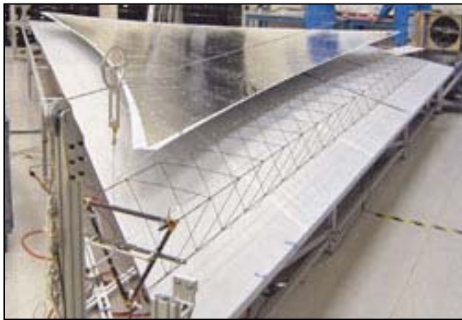
SAILMAST is the thin triangular truss in front of the picture. It is attached to a section of a silver foil solar sail section shown here in a laboratory test. The mast in the picture is 2m (6 ft) long. The Space Technology 8 mission will test the SAILMAST, which is 20 times longer.
