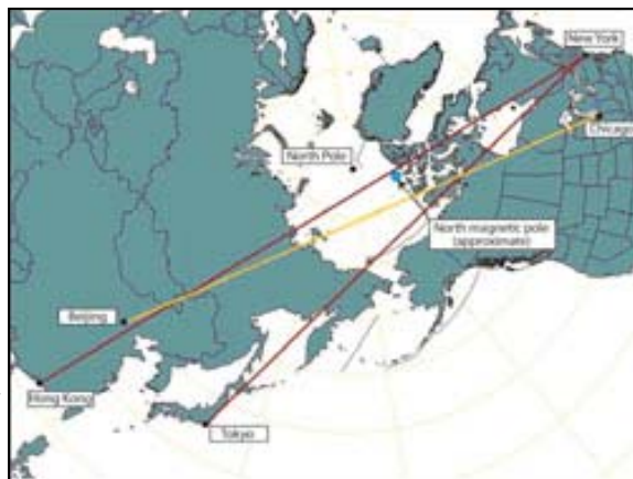
The shortest airline routes from the Eastern U.S. to popular destinations in Asia go very near the magnetic North Pole, where space weather is of greatest concern.
