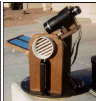
Dobsonian Bino Mount. Capable of handling up to 100mm objective binos.
