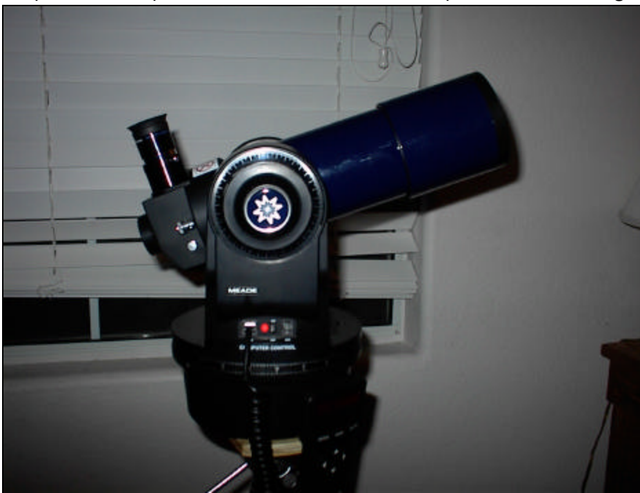
The Meade ETX60-AT. Notice the plywood tripod adapter I made under the base. Quick and simple. The Autostar controller is attached to the base with velcro.
