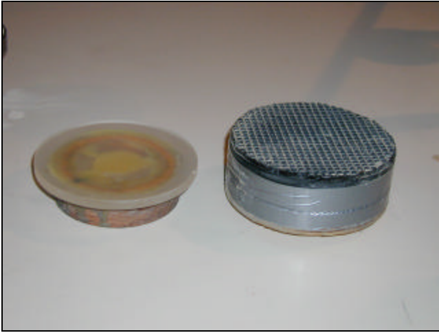
The Pitch Lap used to polish the lens. The lens is on the left, the brown coloring is the Cerium Oxide Compound used to polish the glass.
